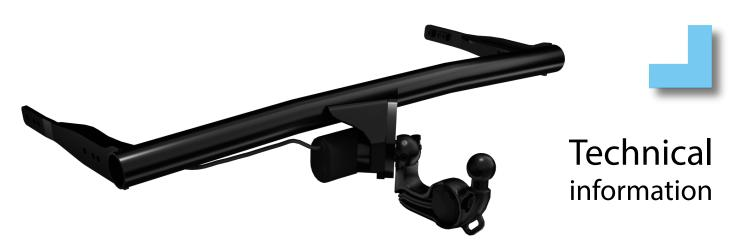
D-value = 10.4 – 12.6 kN Max. trailer weight = 2 500 kg Max. vertical load = 100 kg
